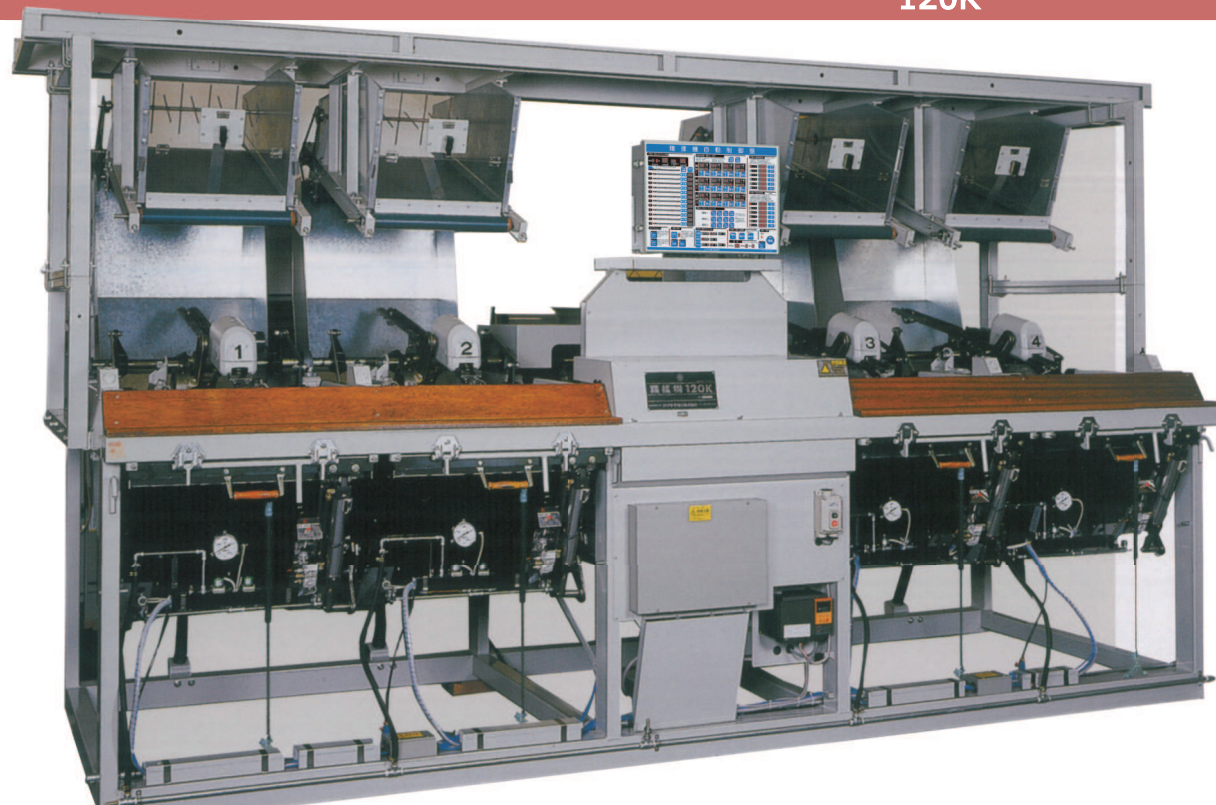
Pressing arm mechanism to roll into round and thin tea leaf shape
