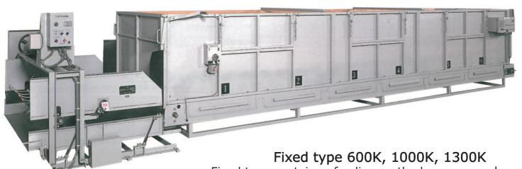
Fixed type container, feeding methods are manual feeding or using a movable fresh leaf feeding conveyor. Automatic removal provided by attaching to a vibrating hopper or untangling unit.
